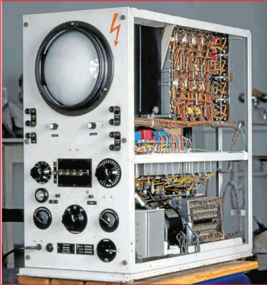
Figure 7. View of the audio-frequency spectrometer near completion of the restoration work. The casing is removed to show the 27-section filter bank and the motor-driven contact array. The modern multi-color parts were required to electronically match the reworked CRT to the original circuit. (original photo)
